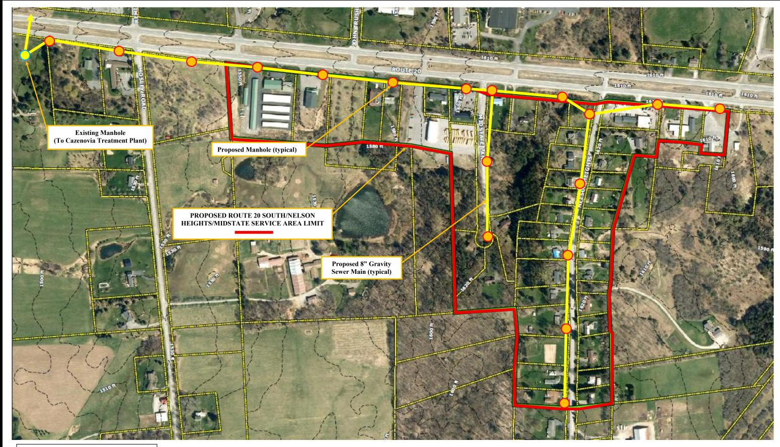
18 Manholes 6,575 Feet of 8" Gravity Sewer Main
