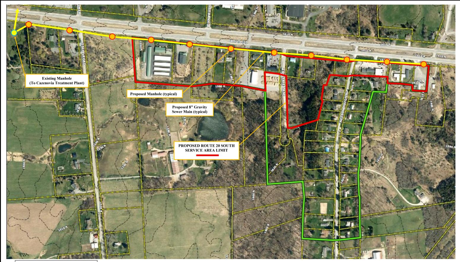
11 Manholes 4,000 Feet of 8" Gravity Sewer Main
